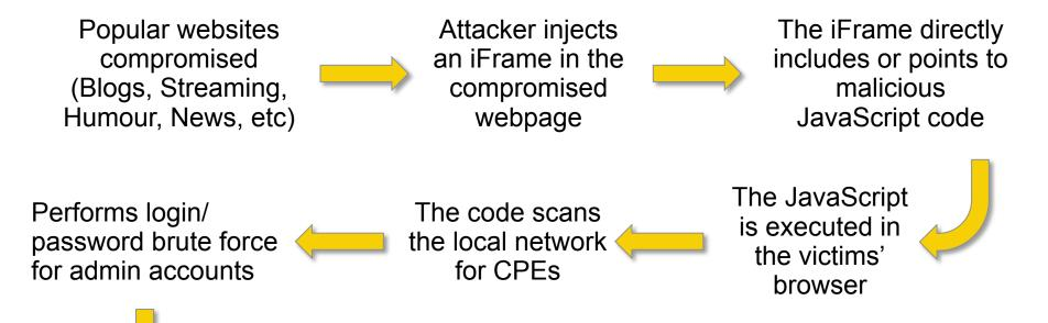
Change the DNS configuration to point name resolution to a rogue DNS server; restart the CPE.
